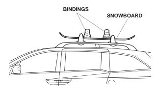
11. If the bindings cannot be positioned between the front and the rear attachments, install the the rear binding behind the rear attachment as shown.
